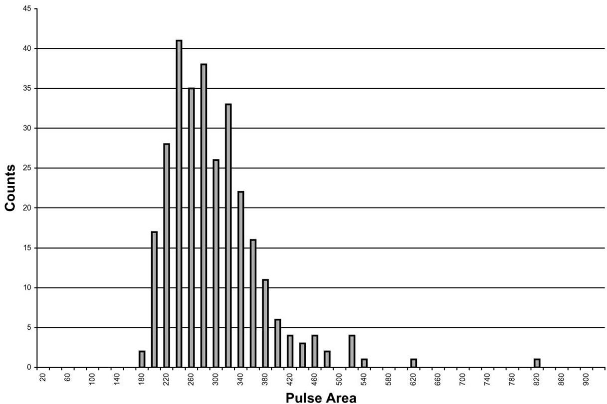
Fig. 1. Pulse-area spectrum of  $75\text{ cm}^3$  dosimeter for 4-MeV incident neutrons.
