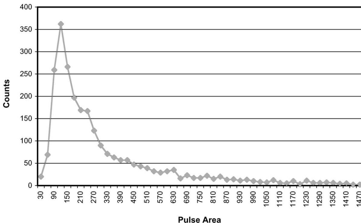
Fig. 3. Pulse-area spectrum for bare  $^{252}\text{Cf}$  source, uncorrected for detector efficiency vs. energy.
