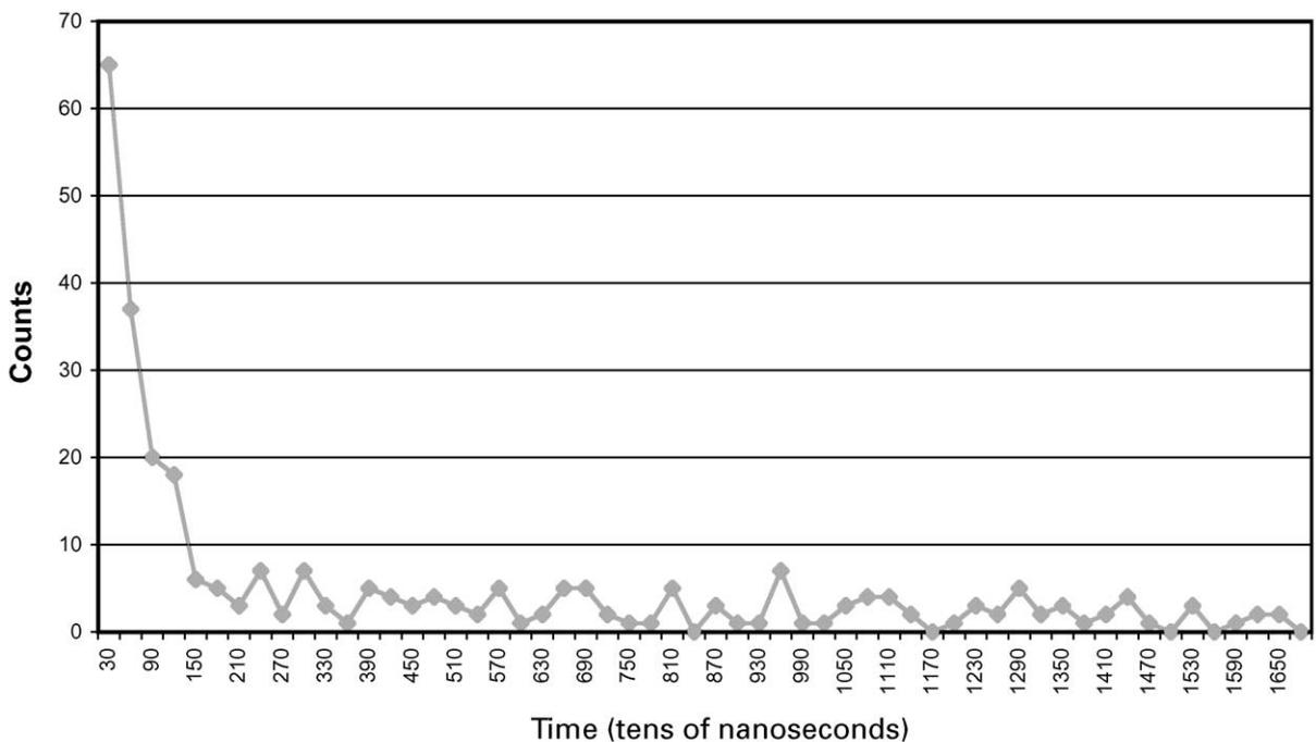
Fig. 2. Time-interval spectrum for 1-cm-thick spectrometer.
